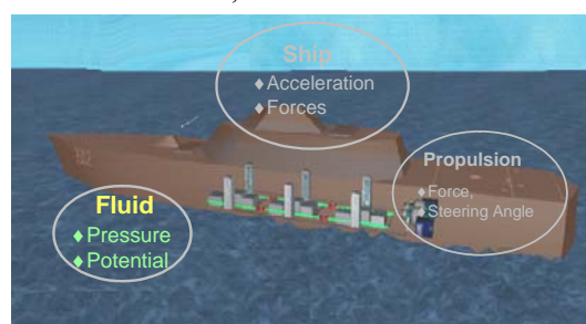
Figure 1 Typical Interacting Components of a Marine Vessel Model
