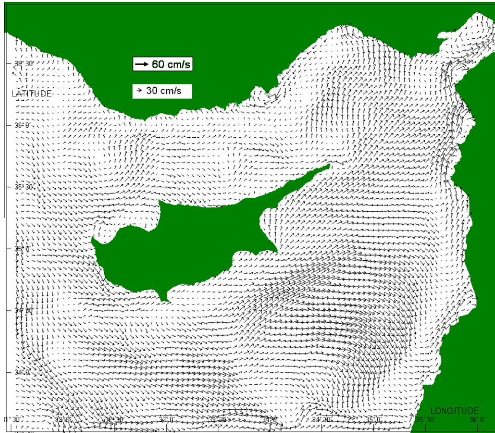
Fig. 6. Surface-currents field for 23 July 2006 at 12:00 from the CYCOFOS forecasting system. Dark arrows represent current directions and intensity in cm/s.
