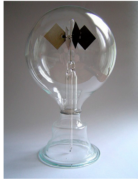
Figure 1. Crookes radiometer. It is made from a glass bulb with low air pressure inside. Within the bulb there is a rotor with several vertical metal vanes, which are polished on one side and black on the other. When exposed to light the vanes turn, the dark sides retreating from the radiation source and the light sides advancing. (Public domain picture.)
